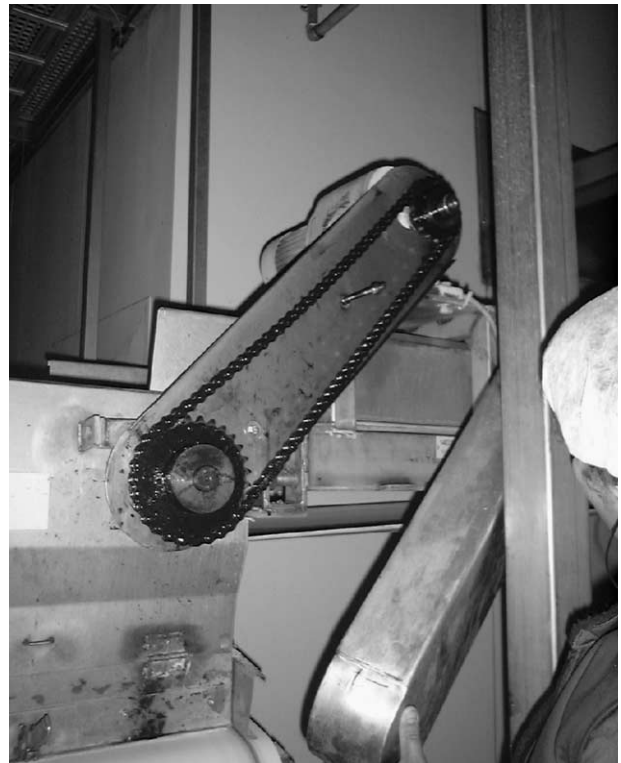
Fig. 5. Open lubrication point: a risk for contamination.
